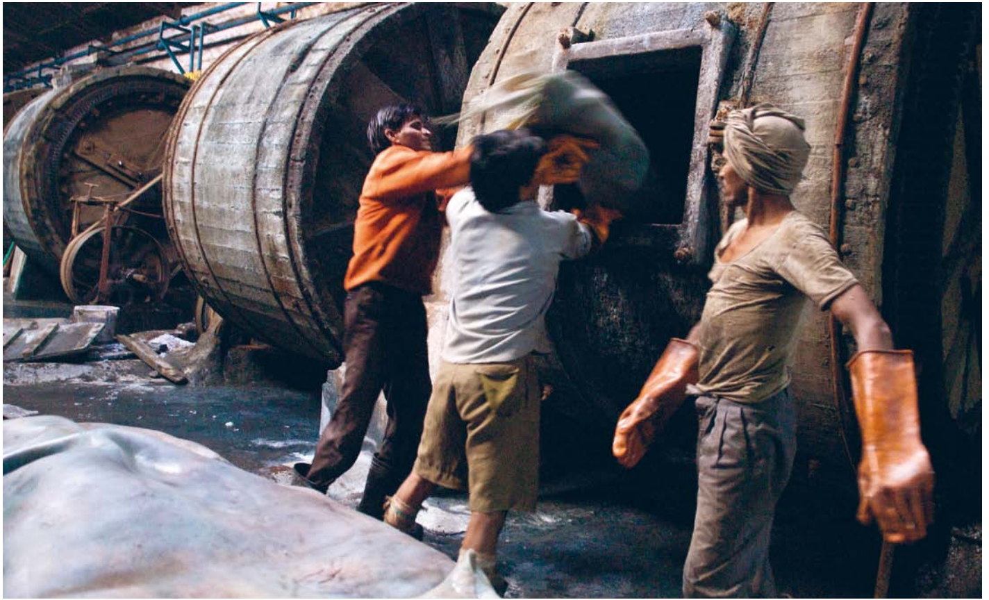
▲ Workers at one of Kanpur's four hundred tanneries, the city's primary industry, load hides into well-used tumblers. Treating leather in this manner is a multi-step process requiring chemicals such as chromium and copious amounts of water. After the water is used, and thus highly polluted to human and animal use, it is more often than not piped back to the Ganges without any treatment.
