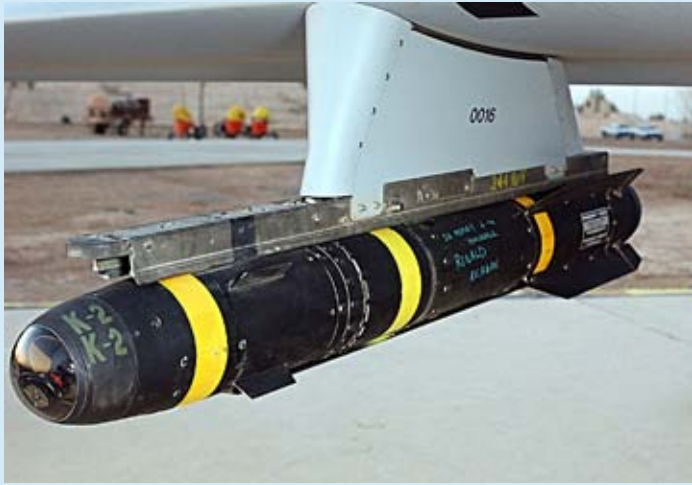
▲ An AGM-114 Hellfire missile hung on the rail of an US Air Force MQ-1L Predator Unmanned Aerial Vehicle (UAV). © TGST Scott Reed, Wikicommons
